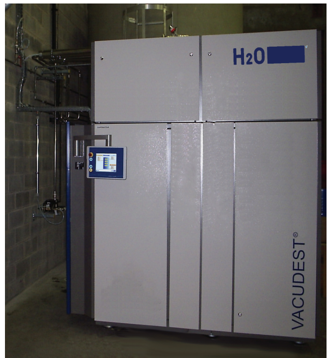
VACUDEST 250 Clearcat for the treatment of degreasing rinsing water
